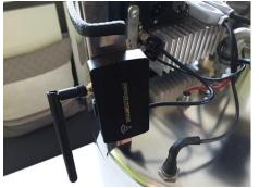
Remove the WLAN module from the carton and clip the module to the side-base on the Braumeister using the clamp on the reverse side of the module. In the beginning, this type of clamp is always very stiff, in order to make sure that module remains tightly clamped to the base. The module is clamped to the side of the controller on the 2001 and 5001 operating models. On the reverse side of the controller on the new 2015 generation, you will find another screw connector next
