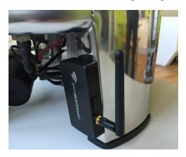
Remove the WLAN module from the protective carton and mount it on a Braumeister base. Plug the cable gland into the free socket on the reverse side of the Braumeister controller and tighten (connect the temperature sensor as well).
