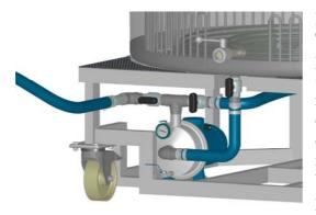
For decanting, use a suitable, clean hose. The hose connection as well as the valve positions can be seen in the figure. (Caution! if the device is not level, the wort runs straight out as soon as the stopcock is opened!). Now you can switch the pump over to manual mode (to change to manual mode, hold down the first and second buttons from the left at the same time) and pump off the wort at your convenience.
