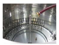
Fill up the kettle with 575 L of brewing water – up to the top mark on the drawbar or alternatively on the filling level sensor. Follow the instructions on the brewing control by acknowledging with ENTER that water has been added. The pump primes itself and the programmed mashing temperature is started.
