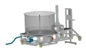
Place the Braumeister in the cleaning position by cranking down the rear support and thus tilt the Braumeister. Connect the hose to the waste water system and position the valves as per the figure on the left. Now you can clean the Braumeister from the top with a suitable brush and water and at the same time pump the waste water (in manual mode) away into the drain.
