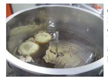
Continue with START, to start boiling the hops. Do not put the lid on. Avoid boilover. Add the first hops (350g) 10 min after start of boiling. Do not put the lid on even when boiling the hops. Vapours must be able to escape. Top up the evaporated water or adjust the original gravity. The last hop addition (150g) takes place 10 min before flame out.
