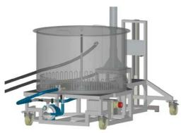
To do this, connect up the hoses and position the valves as per the figure on the left. With a low pump speed (dial position 6-8) you achieve a smooth rotation of the wort in the kettle. Caution! The pump only switches back on at 86°C. In addition, the rotation helps to optimise cooling. In this case, a cooling time of roughly 90 min is required to go from 100°C down to 20°C.
