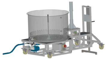
Immediately after brewing, it is best to place the Braumeister in the cleaning position (see figure, left) and to pump off all the fine solids diluted with water. Observe the correct valve positions.
