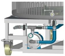
First of all the kettle is filled with 575 L of brewing water (up to the top mark). At this point, the malt pipe is not yet installed. The marks on the drawbar show the filling levels for 425 L, 500 L and 575 L. For the valve positions for the heating phase, please see the figure on the left.
