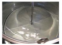
Once the mashing temperature is reached, a warning tone sounds which you acknowledge with ENTER. Now insert the malt pipe (with seal fitted, facing downwards). Take care that the seal with the malt pipe is centred and is sitting absolutely level on the kettle bottom. Insert the first sieve insert as far as the bottom edge.
