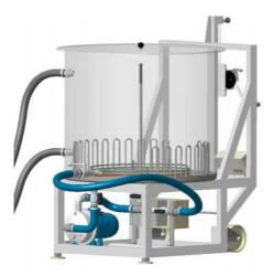
To do this, connect up the hoses and position the valves as per the figure on the left. With a low pump speed (dial position 6-8) you achieve a smooth rotation of the wort in the kettle. Caution!: the pump only switches back on at  $86^{\circ}$ C. In addition, the rotation helps to optimise cooling. In this case, a cooling time of roughly 50 mins. is required to go from  $100^{\circ}$ C down to  $20^{\circ}$ C.
