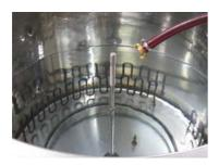
Fill up the kettle with 230 l brewing water – up to the top mark on the drawbar or alternatively on the filling level sensor.
