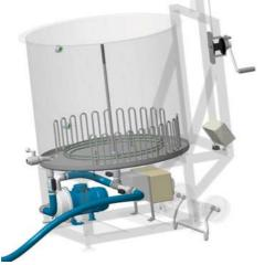
Place the Braumeister in the cleaning position by folding down the rear supporting bracket which holds the Braumeister inclined. Connect the hose to the waste water system and position the valves as per the figure on the left. Now you can clean the Braumeister from above with a suitable brush and water and at the same time pump the waste water (in manual mode) into the drain.
